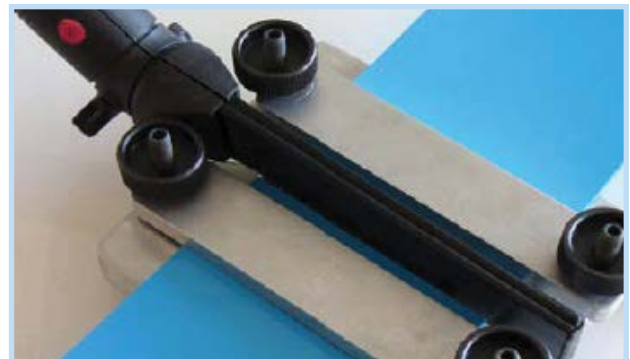
Welding narrow flat belts with Pliers P-200
