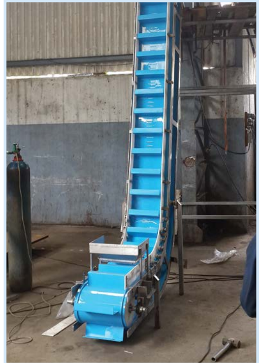
Fixed conveyor side wall
