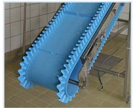
SuperDrive™ with Sidewalls and Special Flights
