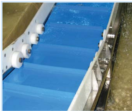
SuperDrive™ with Flights Working under Water
